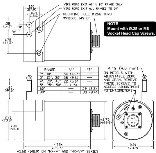
Note: Dimensions in brackets are millimeters.
