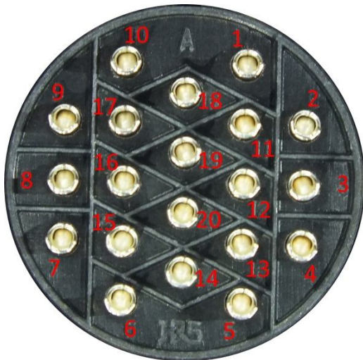
1 Pin Connections, rear of 20-way Hirose
