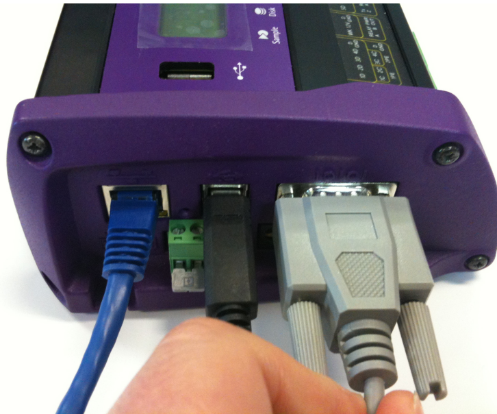
Figure 1 – Serial RS-232 connection to the dataTaker DT80
