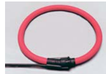
FX3000 10 amps to 3000 amps AC FX5000 100 amps to 5000 amps AC Both models: Accuracy 2%, Size 24" long for conductors up to 7.5" diameter
